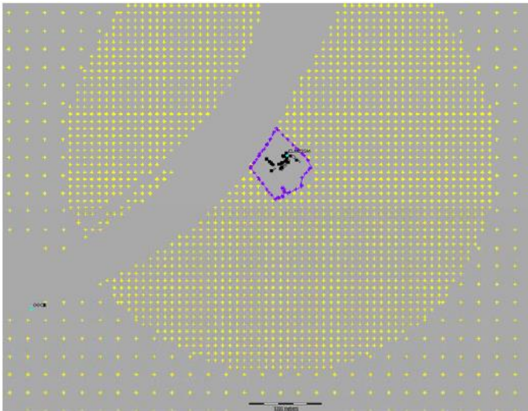
Figure 19: Receptor Grid for the Daviess County Area. Source, Zoomed in Around the Elmer Smith Station area: “Air Dispersion Modeling Report: Elmer Smith Station, Owensboro, Kentucky SO 2 Designation Analysis Data Requirements Rule, Revision 1,” prepared by Elmer Smith Station, April 28, 2016.
