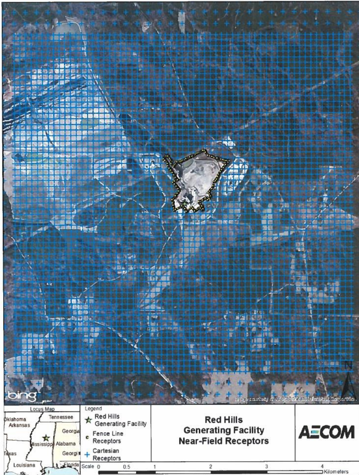
Figure 4. Receptor Grid for the Choctaw County, Mississippi Area. Source: 1-Hour SO 2 NAAQS Designation Modeling Report prepared for Mississippi, December 2016.
