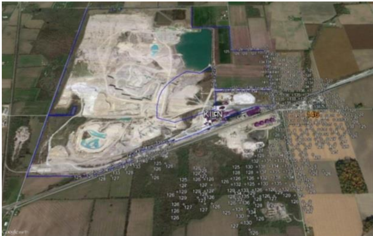
Figure 11-6: Predicted 99 th Percentile Daily Maximum 1-Hour SO 2 Concentrations Averaged Over Three Years for the Carmeuse Lime Area of Analysis
