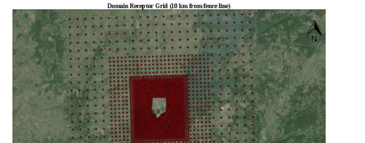
Figure 15. Domain Receptor Grid (10 km from Fence Line) for AEP/PSO Northeastern Power Station
