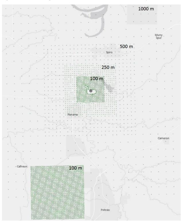
Figure 23. Domain Receptor Grid (10 km from Fence Line) for AES Shady Point
