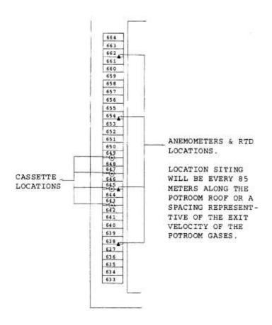
Figure 14A-3. Conceptual side view of positions of cassettes, anemometers, and RTDs in a typical half of a potroom.
