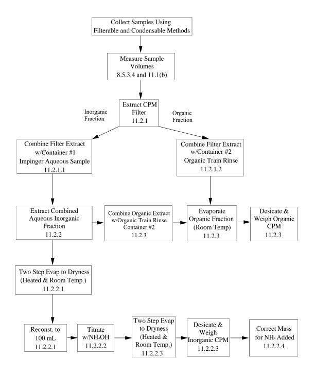
Figure 7. CPM Sample Processing Flow Chart
