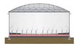
For example, a 120-foot diameter tank located in Houston, a similar climate to St. James, storing gasoline with an RVP of 10 and 24 cycles per year is estimated to emit 2,986 lbs./year less VOC if equipped with a self-supported geodesic roof compared to a column-supported cone roof.<sup>154</sup>
