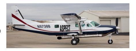
ASPECT consists of a suite of sensors and software mounted in a fixed wing single engine aircraft and uses the principles of remote hazard detection to image, map, identify, and quantify chemical vapors and deposited radioisotopes. It provides first responders – emergency workers on scene -- with actionable information on the situation.
