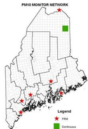
A continuous PM<sub>10</sub> TEOM monitor is operated in Presque Isle as part of the control strategy for the historically high PM<sub>10</sub> levels there. The PM<sub>10</sub> TEOM provides hourly data used by city officials to determine when high levels are occurring and whether street sweeping or other control strategies need to be implemented.
