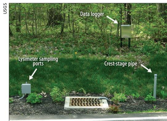
Figure 11. Roadside rain garden in Cuyahoga County is monitored for its effectiveness in absorbing stormwater.
