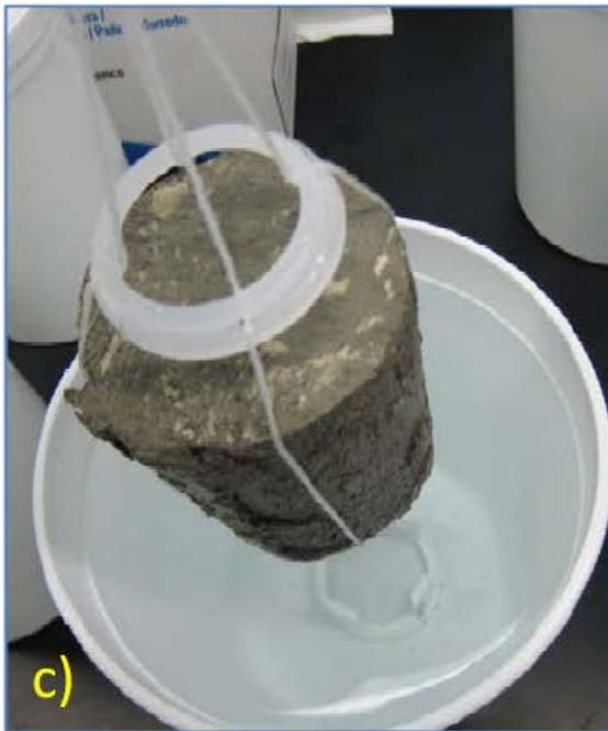
c) Removing Sample for Exchange
