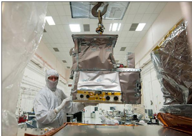
IASI - Infrared Atmospheric Sounding Interferometer Michelson interferometer 236 kg. 210 W 12 km FOV at nadir, non-contiguous Launched on MetOp-a in 2006 and MetOp-B in 2012
