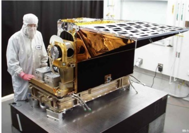
IASI - Infrared Atmospheric Sounding Interferometer Michelson interferometer 236 kg. 210 W 12 km FOV at nadir, non-contiguous Launched on MetOp-a in 2006 and MetOp-B in 2012
