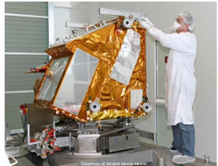
CrIS - Cross-track Infrared Sounder Michelson interferometer 85 kg. 110 W 3x3 14 km FOVs at nadir, contiguous Launched on S-NPP in 2011
