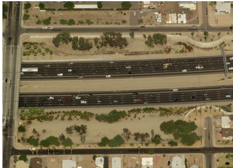
Figure 10. Oblique aerial photo of the I-10 at 12 th Street. Note there is a sound wall on the north side of the freeway, but not the south side. There is a steep slope on the south side, however.
