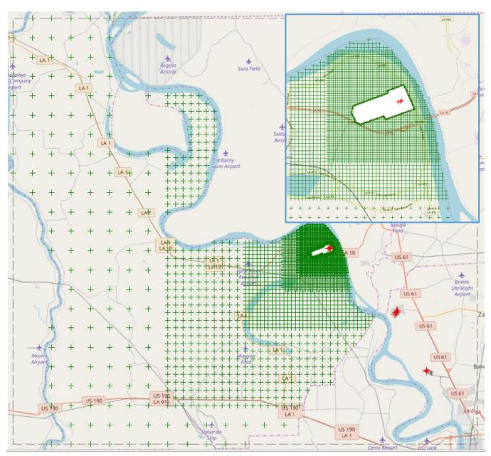
Figure 3: Area of Analysis and Receptor Grid for the Pointe Coupee Area
