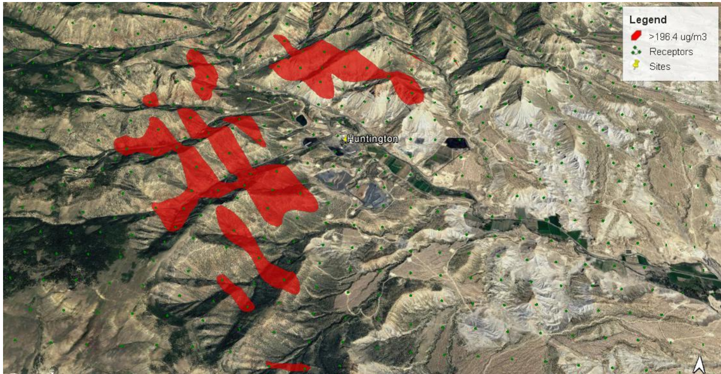
Figure 11. Figure generated by the EPA using the SC Hunter Simulation output files provided by Sierra Club. The results in the figure show the cumulative impacts from the Hunter and Huntington power plants and include background concentrations. The results are the same as Figure 9 but focuses on the area around the Huntington Power Plant. Red shaded areas represent receptors violating the NAAQS.
