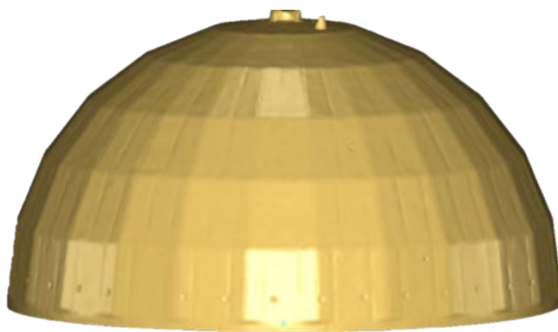
Upper Dome Diagram depicting how flat plates were used to create upper dome
