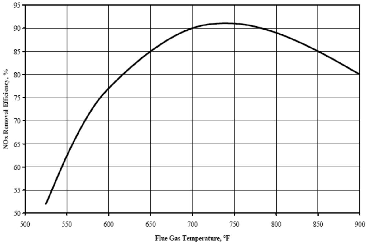
**Figure 2.2: NO<sub>x</sub> Removal versus Temperature [50]**
