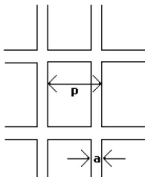
**Figure 2.5: Pitch for a Honeycomb Catalyst Configuration**
