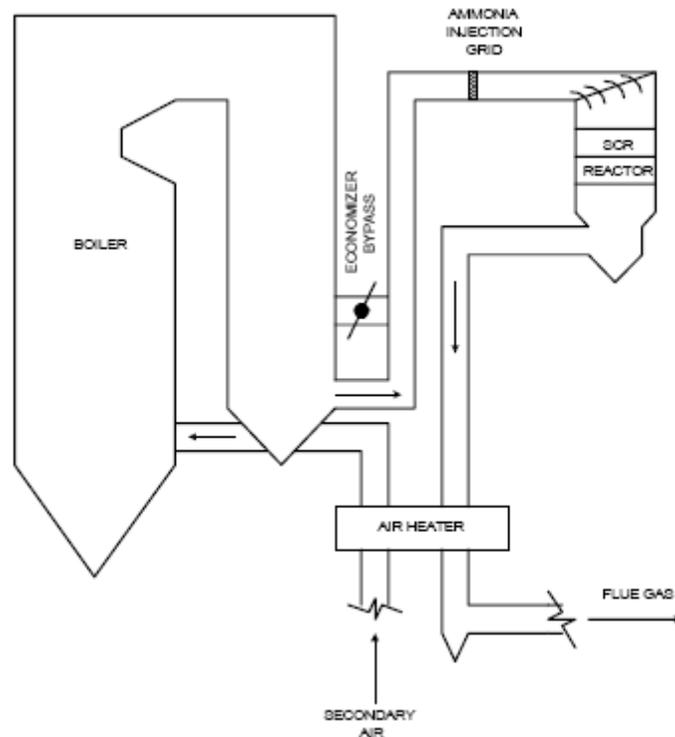
**Figure 2.7: High-Dust SCR Arrangement [46]**
