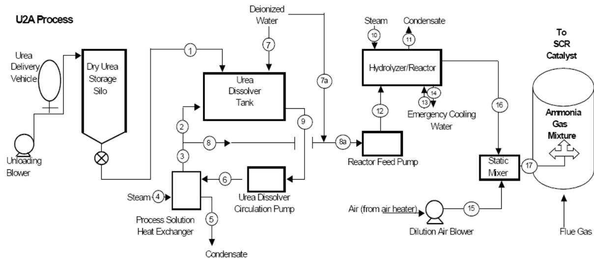
**Figure 2-11: Urea-Derived Ammonia Production System Using U2A system [84]**
