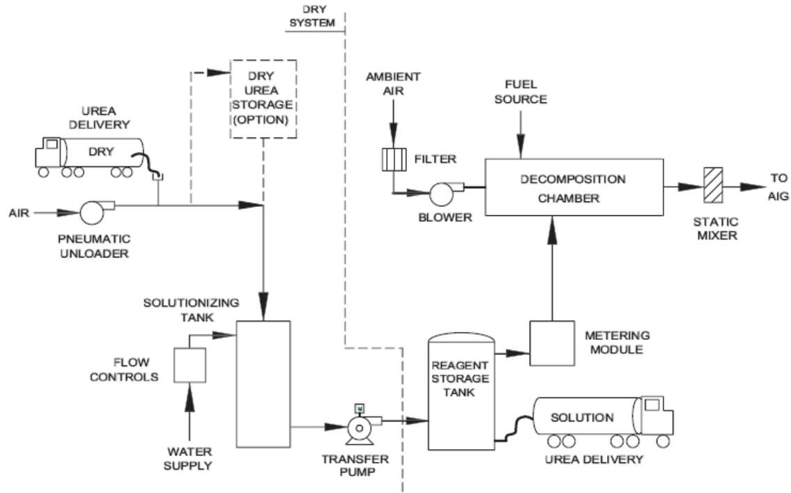
**Figure 2.12: Urea-Derived Ammonia Production System Using NO<sub>x</sub> ULTRA System [87]**
