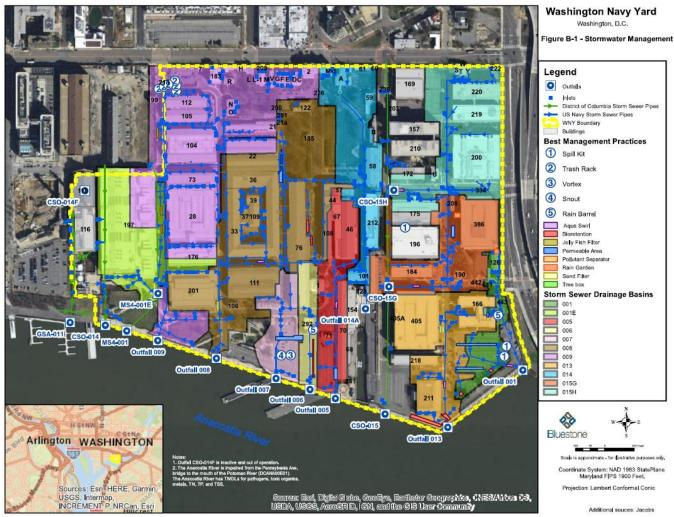
Map of the Washington Navy Yard outfalls and stormwater BMPs. Note, Outfall 014F has been permanently eliminated. Image borrowed from the permittee's 2020 Stormwater Pollution Prevention Plan.
