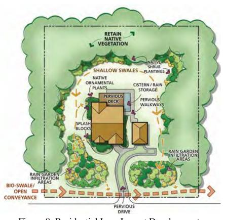
Figure 8: Residential Low-Impact Development Low impact development (LID) practices, many of which are shown above, reduce stormwater runoff and reduce the need for large regional stormwater treatment systems.
