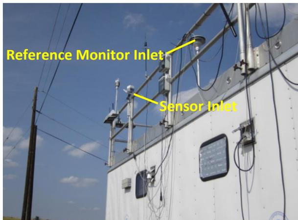
Example of sensor inlet located near reference monitor inlet.
