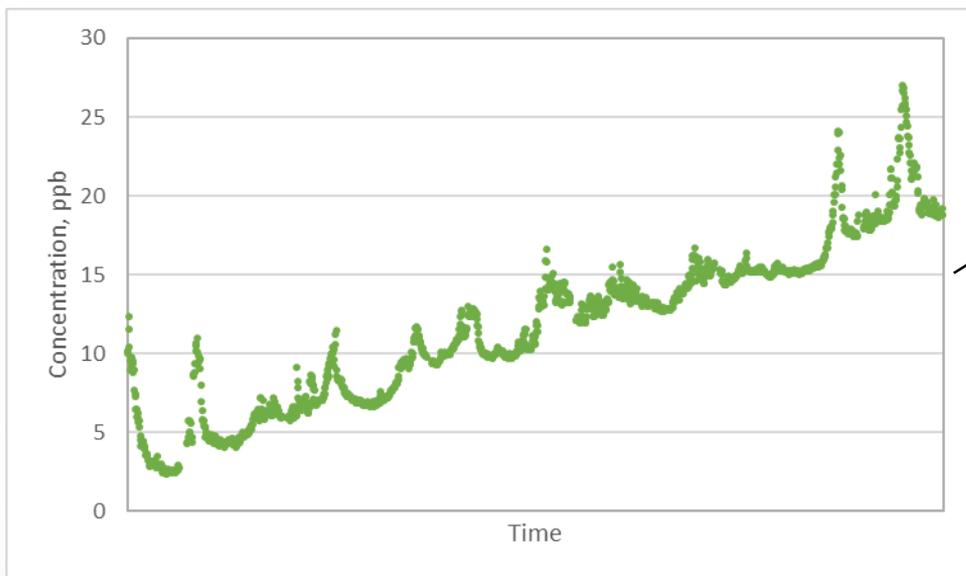
Concentrations reported by the sensor are increasing gradually over time. Looks like the sensor's response is drifting.
