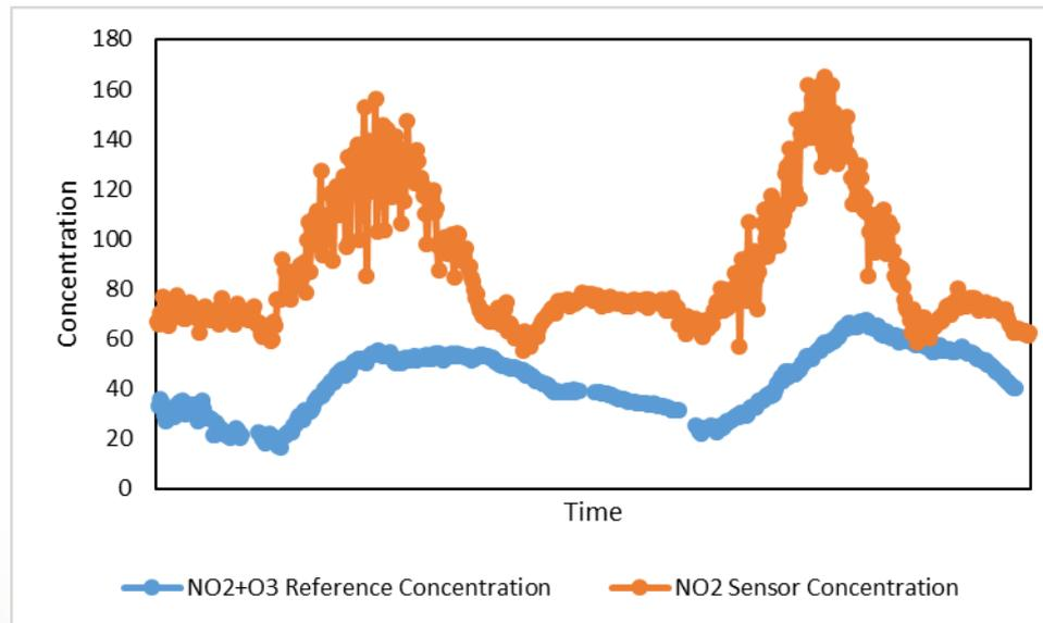
The sensor is supposed to be measuring NO<sub>2</sub>, but it's reporting concentrations higher than the combined reference NO<sub>2</sub> and O<sub>3</sub> concentrations. Could be a measurement interference.
