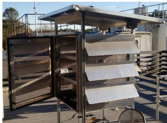
Example of a custom-made weather shelter for sensor evaluation.
