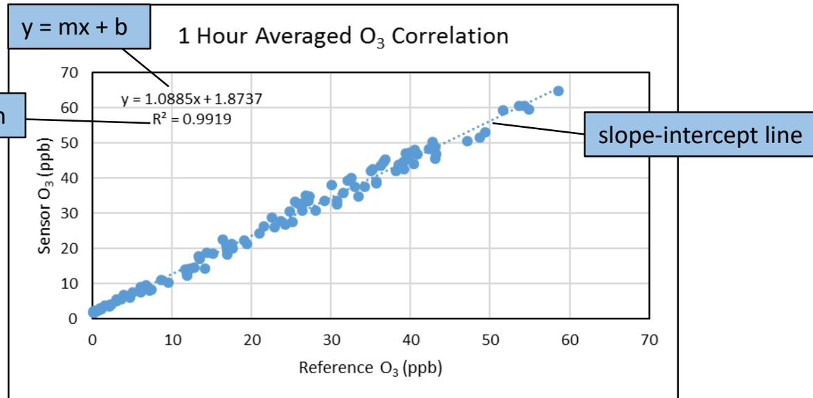
The line going through the data is called the “slope-intercept” line and is represented by the equation  **$y = mx + b$** . This equation is a statistical means of comparing the sensor data with the reference data. The **coefficient of determination**, represented by  $R^2$ , is a measure of how close the data are to the slope-intercept line.
