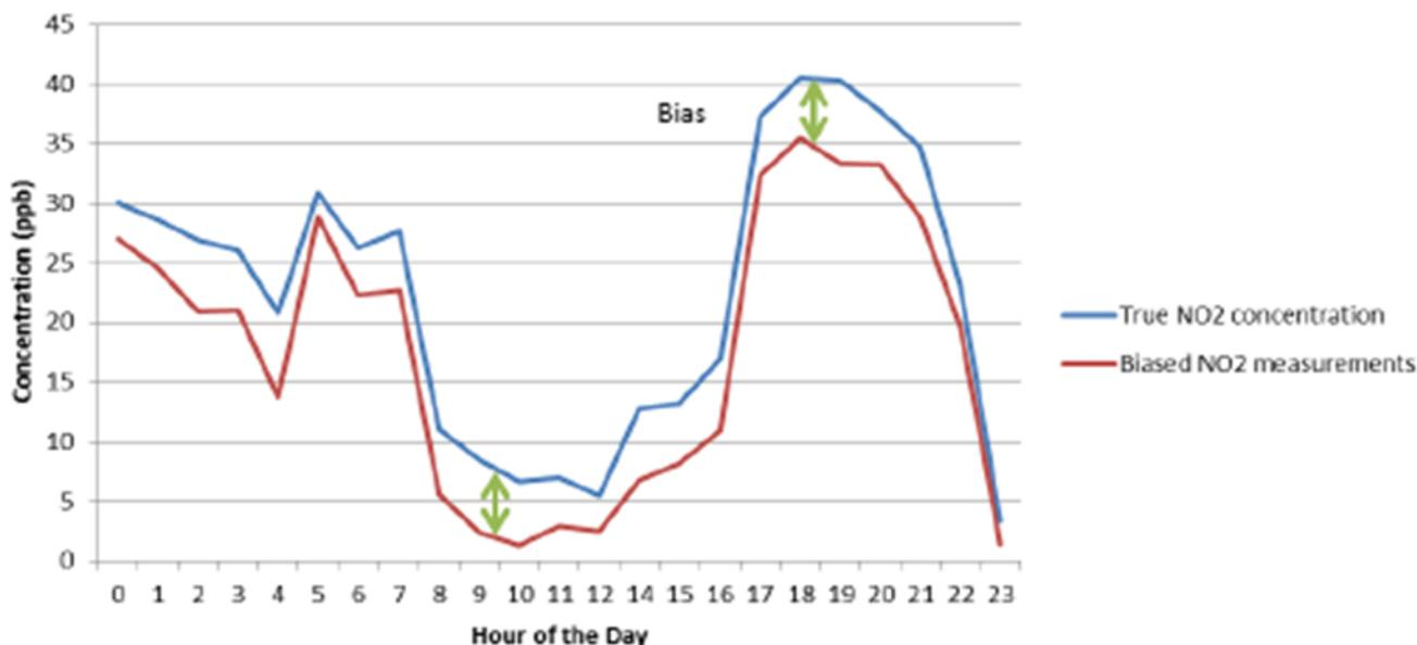
Comparison of a true value of NO2 and biased measurements of NO2.
