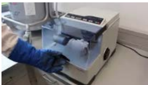
Figure 29. Retsch Cryomill uses liquid nitrogen to embrittle polymer samples.
