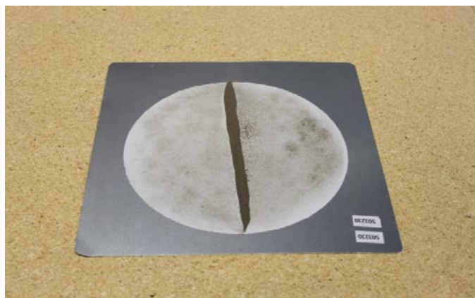
Figure 82. The dust particles form a line after the aluminum sheet is folded into the U shape. The unfolded panel shown in this picture is a thin aluminum plate instead of 4-mil aluminum foil.
