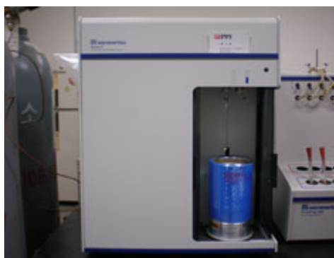
Figure 31. Micromeritics Gemini V series BET surface area analyzer
