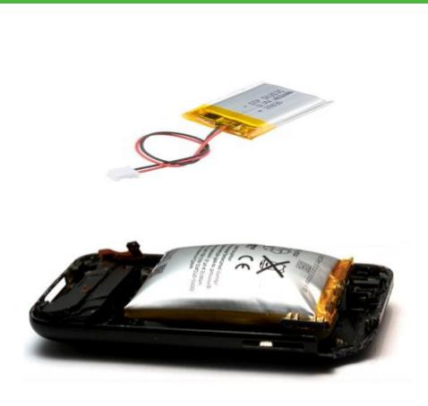
Pouch lithium polymer battery is favored for its lightness but is damaged easily.
