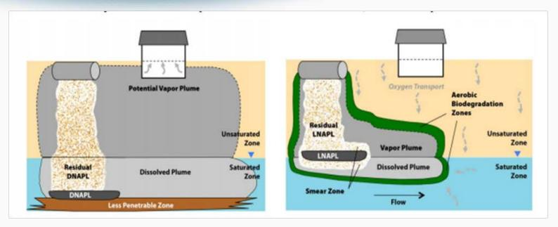
Chlorinated Solvent (left) petroleum (right) are distinguished by prospects for biodegradation
