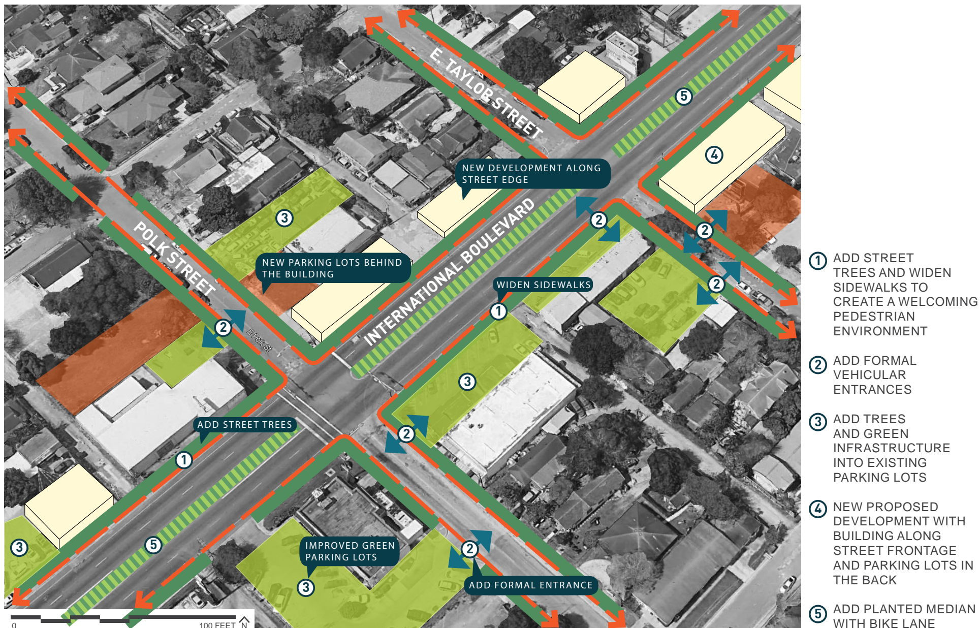
FIGURE 64 Best Practices for Commercial Developments along Highways. This diagram shows best practices which could occur at site 3B. It focuses on shifting store frontages to the street edge and adding street trees and buffered planting. Parking lots move behind buildings and commercial entries are shifted to side streets where possible.
