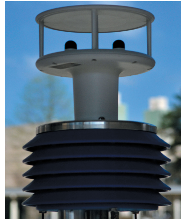
SPod air sensor device.
