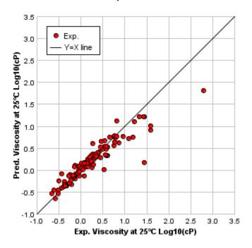
Figure 4.12.1. Experimental vs predicted values for the viscosity test set
