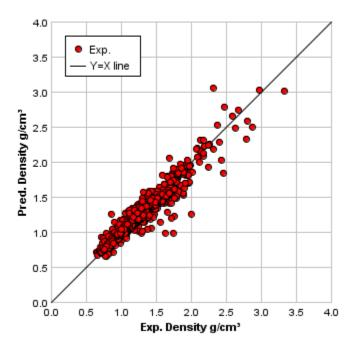
Figure 4.9.1. Experimental vs predicted values for the density test set
