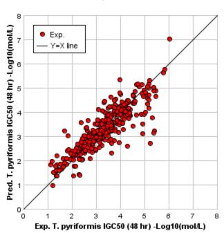
Figure 4.3.1. Experimental vs predicted values for the *T. pyriformis* IGC<sub>50</sub> test set
