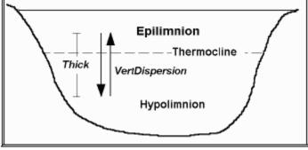
Inflow of water (and the loadings within that waterbody) can be routed to a specific vertical segment, as can the outflow of water.
