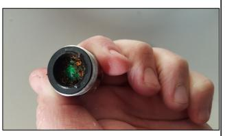
Picture of an aerator with particulate
