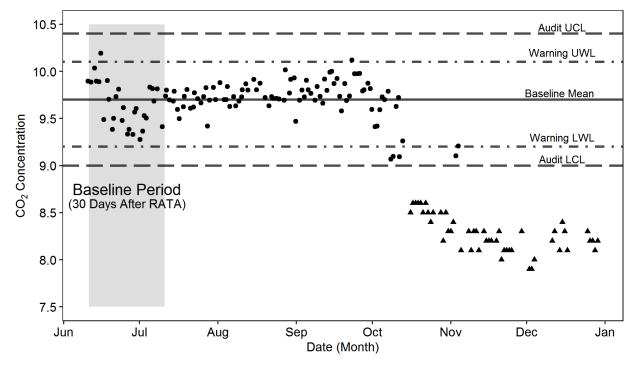
Figure 4. Typical CO<sub>2</sub> control chart
