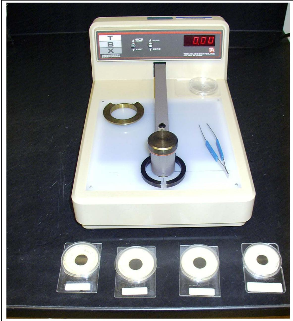
**Figure 2-2.** Tobias TBX-10 Densitometer with Calibration Standards
