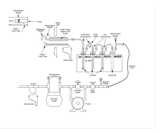
Figure 8-1. Sulfuric Acid Sampling Train
