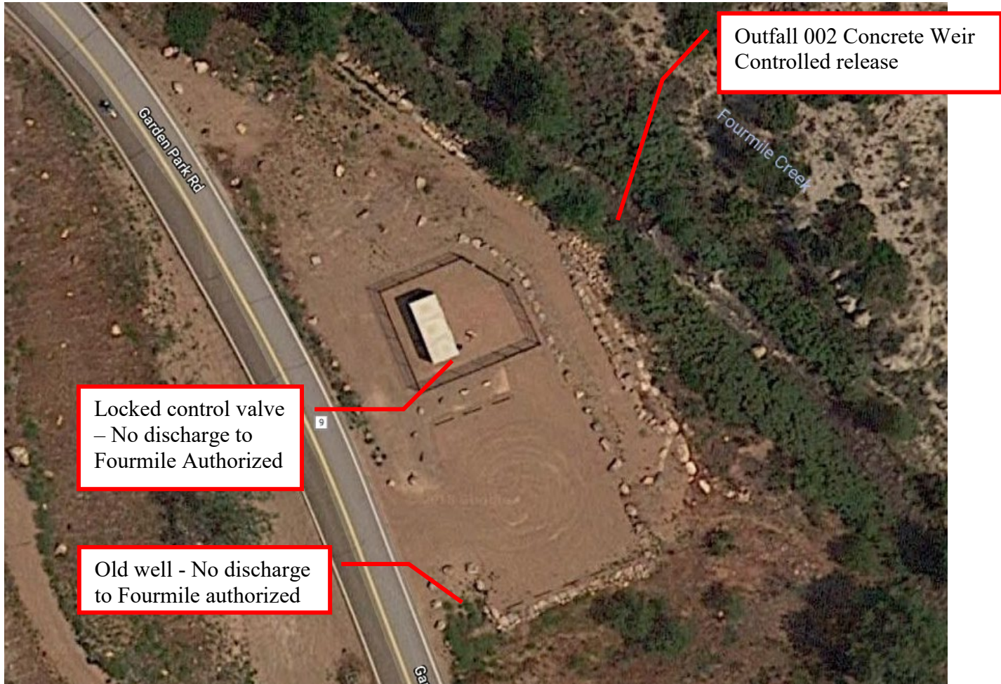
Figure 1 - Aerial image of Park Center Well site.
