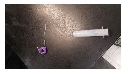
2. Place the coil in the beaker of water and draw in about 5 mL of water.
