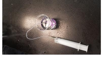
3. Take the coil out of the water and pull up some air.
