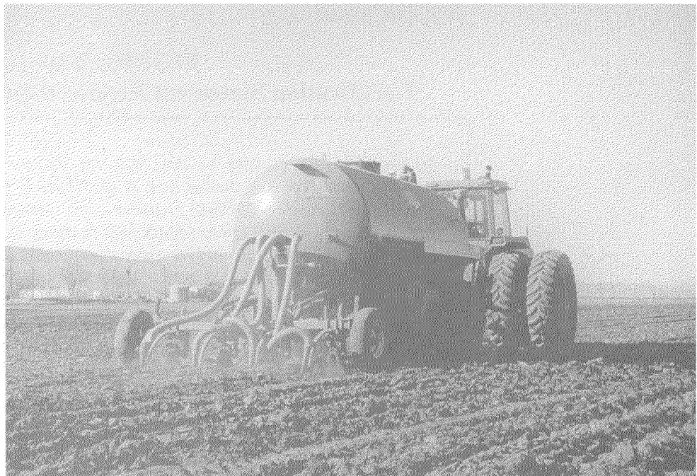
Anaerobically digested biosolids from Los Angeles are injected into the soil in California.
