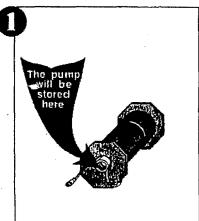
Unpack the components of the Redi-Fio2 system. The MP1 pump will be packed in the center of the motor lead roll.
