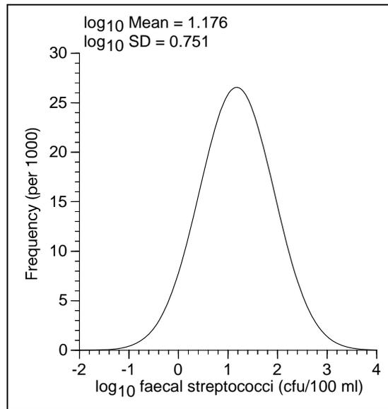
**Figure C-1. A Probability Density Function of Faecal Indicator Distributions Measured at a Recreational Water Showing Probability of Exposure (Y Axis) versus Log10 Faecal Streptococci Concentration (later termed enterococci).**
