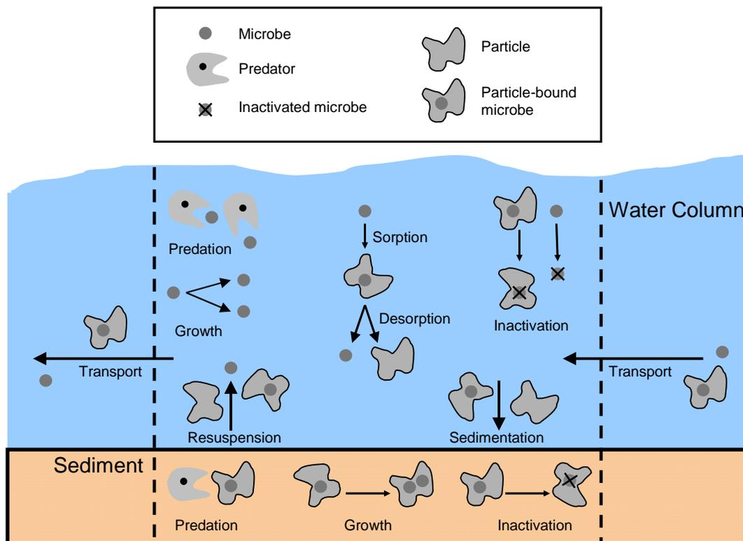
**Figure 5. The Possible Fates of Microbes (Fecal Indicators and Pathogens) in Environmental Water and Sediment** (the fate of nucleic acids may be different; this figure does not include those sources). SOURCE: Adapted from Olivieri et al. (2007).
