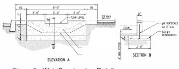
Figure 9 - Weir Construction Detail
