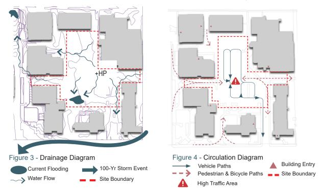
observations of the site recorded the interactions that occurred between pedestrians and vehicles, and what routes were necessary for maintaining the necessary functions of access and parking. (Figure 4) The following diagram shows the dangerous context occurring through the center of the parking lot along the unofficial pedestrian corridor.
