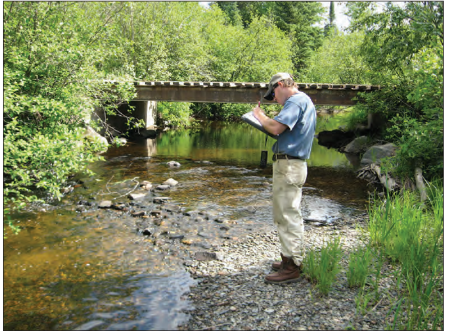
Figure 6. U.S. Geological Survey hydrologic technician examining low-water control downstream of bridge at USGS streamgage 04043126 prior to ecological sampling. (Photograph by J.A. Wilkinson, U.S. Geological Survey)
