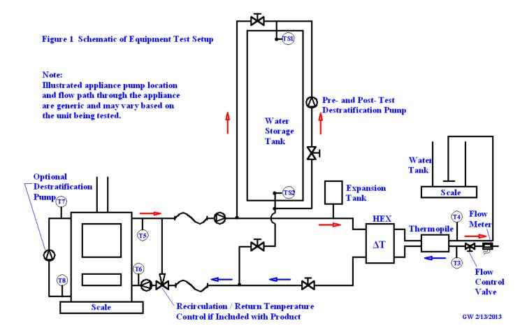
Figure 2. Schematic of Test Equipment Set-up
