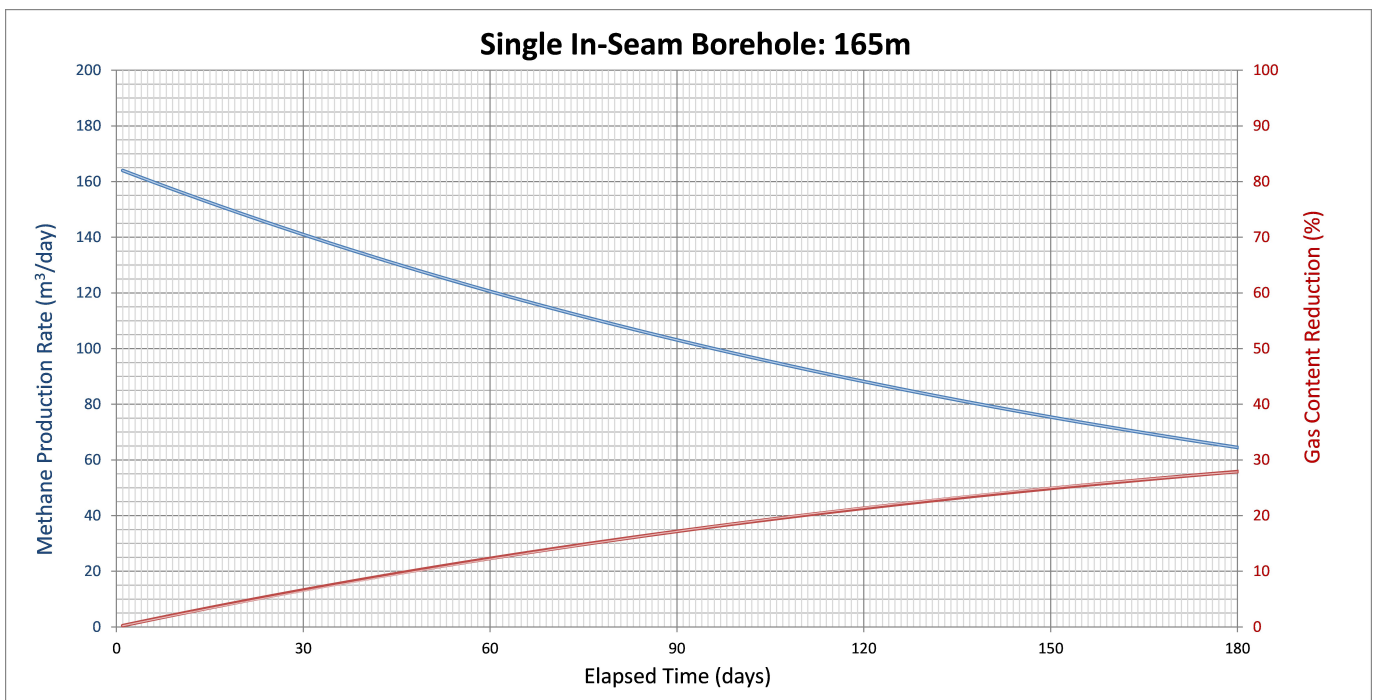
Figure 3-3: Projected gas production and gas content reduction from a single cross-panel borehole in the No. 2 coal seam.
