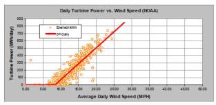
Figure 30: Daily Turbine Power vs. NOAA-AMA Wind Speed
