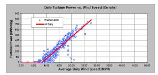
Figure 31: Daily Turbine Power vs. On-site Wind Speed
