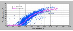
Figure 29: Hourly Turbine Power Bin Analysis
