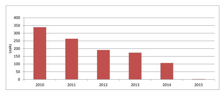
Leak Per Year: The AMRP reduced methane leaks from mains dramatically.
