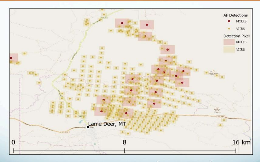
Each detection assigned square area (0.14 km<sup>2</sup> VIIRS or 1 km<sup>2</sup> MODIS) Detection rectangles formed from scan and track sizes of satellite pixel Convex hulls from detection clusters joined to form "**fire polygon**"
