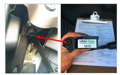
Mini-logger that fits on the in-cab J1939 connector, to acquire vehicle diagnostic data
