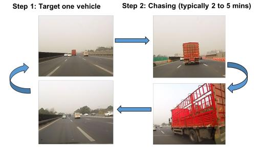
Step 3: finish chasing, pass and then measure road background (~1 min)
