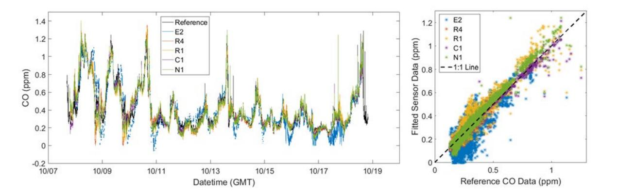
Here is a co-location of 5 Pods (equipped with electrochemical CO) in LA
