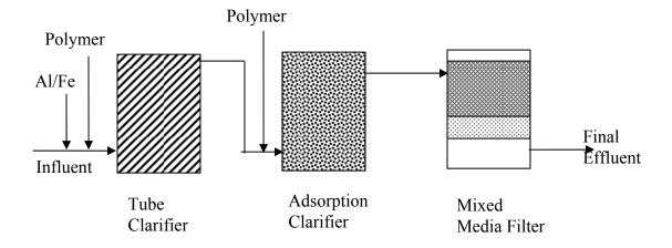
Figure 2-21. U.S. Filter Trident process.
