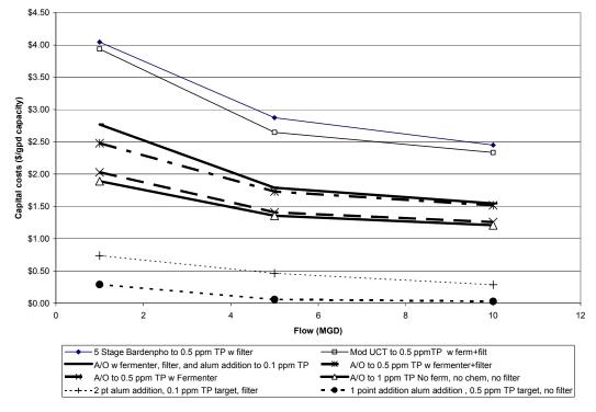
Figure 4-11. Capital costs for expansion phosphorus removal technologies.
