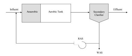
Figure 2-15. A/O (Phoredox) process.
