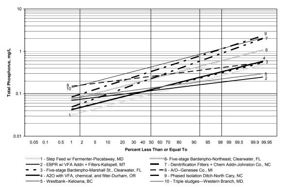
Figure 2-36. Monthly frequency curves for TP removal—mid-range removal.
