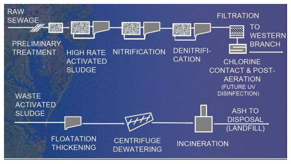
Figure 1. Western Branch WWTP process flow.
