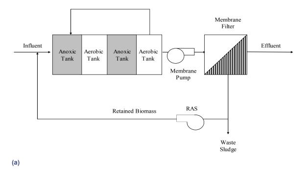
Figure 2-9. MBR process. (a) External filter in lieu of clarifier
