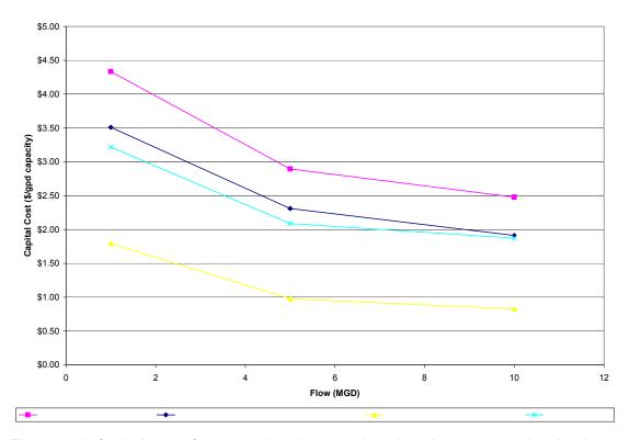
Figure 4-21. Capital costs for expansion nitrogen plus phosphorus removal technologies.
