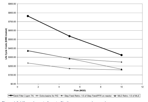
Figure 4-6. Life-cycle costs for retrofit nitrogen removal scenarios.
