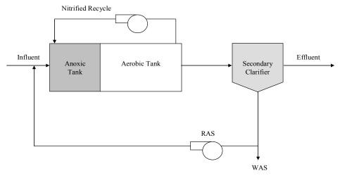
Figure 2-3. Modified Ludzack-Ettinger process.
