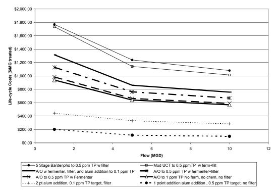
Figure 4-12. Life-cycle costs for expansion phosphorus removal technologies.
