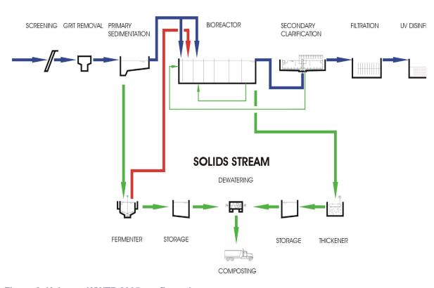
Figure 3. Kelowna WWTP 2005 configuration.
