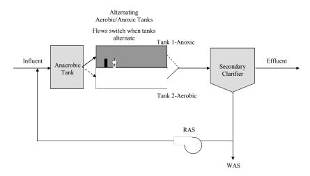
Figure 2-28. Biodenipho (phased isolation ditch) process.
