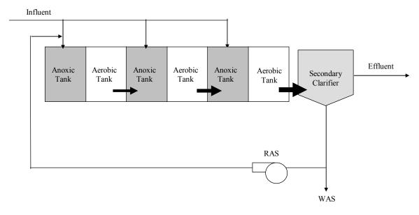
Figure 2-10. Step-feed activated sludge process.
