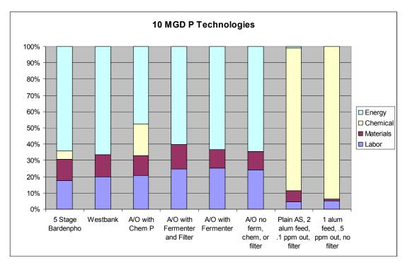
Figure 4-14. Component percentages of total O&M costs for 10 MGD expansion phosphorus removal technologies.
