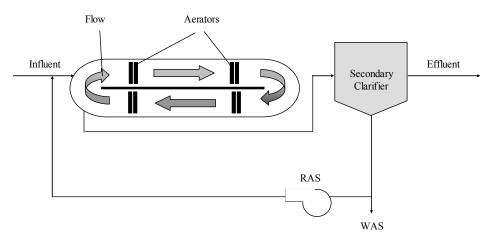
Figure 2-6. Oxidation ditch process.
