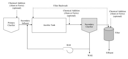
Figure 2-17. Phosphorus chemical/filter process.
