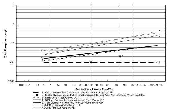
Figure 2-35. Monthly average frequency curves for TP—low-end removal.
