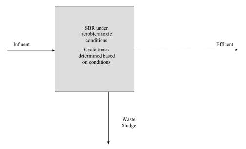
Figure 2-13. Sequencing batch reactor.
