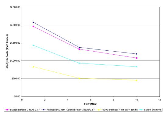
Figure 4-23. Life-cycle costs for expansion nitrogen plus phosphorus removal technologies.
