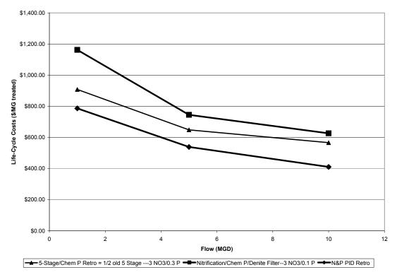
Figure 4-9. Life-cycle costs for retrofit nitrogen plus phosphorus removal technologies.
