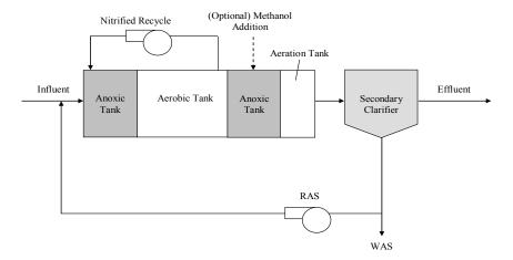
Figure 2-5. Four-stage Bardenpho process.
