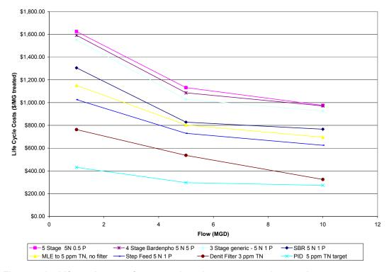
Figure 4-17. Life-cycle costs for expansion nitrogen removal scenarios.
