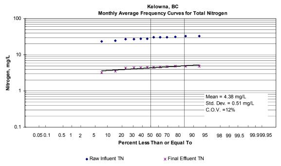
Figure 4. Monthly frequency curves for effluent TN.
