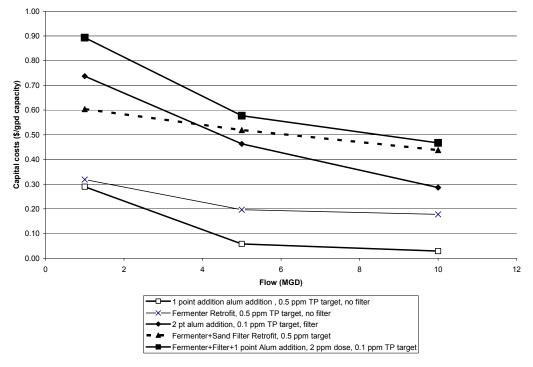
Figure 4-2. Capital costs for retrofit phosphorus removal technologies (\$ per gpd capacity).
