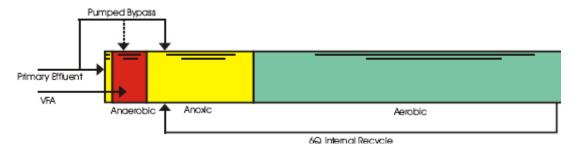
Figure 2. The Westbank three-stage process.
