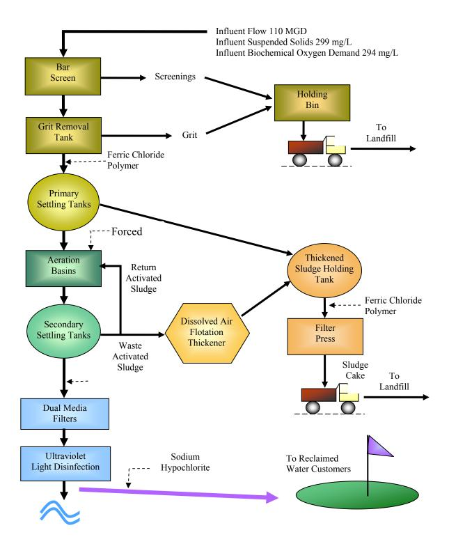
Figure 3. Clark County WRF CP flowsheet schematic.
