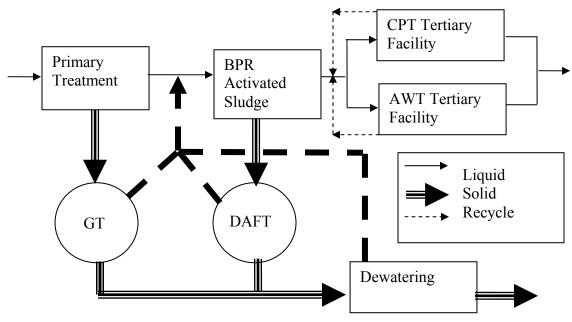
Figure 1. Plant flow schematic.
