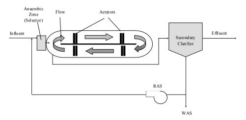
Figure 2-16. Oxidation ditch with anaerobic zone.
