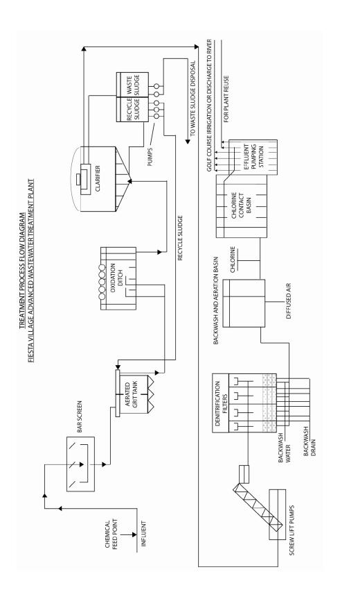
Figure 1. Treatment process flow diagram Fiesta Village Advanced Wastewater Treatment Plant.
