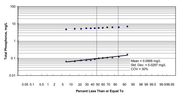
Figure 3-21. Clark County Water Reclamation Plant, Las Vegas, Nevada: Monthly average frequency curve for TP.
