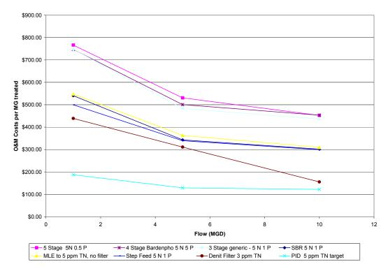
Figure 4-16. O&M costs for expansion nitrogen removal scenarios.
