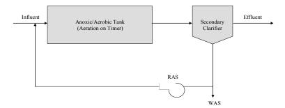
Figure 2-4. Cyclically aerated activated-sludge process.
