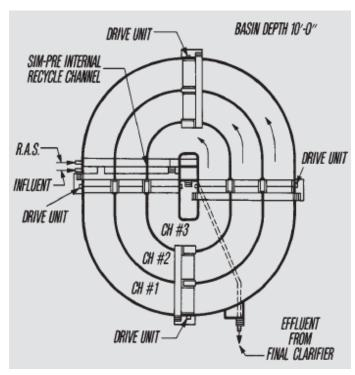
Figure 2-32. Concentric oxidation ditch.
