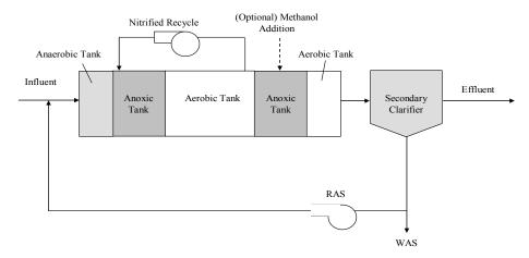
Figure 2-23. Five-stage modified Bardenpho process.
