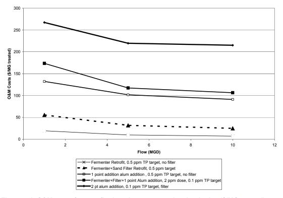
Figure 4-1. O&M costs for retrofit phosphorus removal technologies (\$/MG treated).
