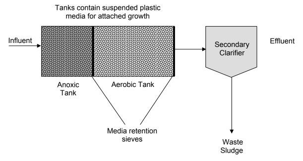
Figure 2-8. Moving-bed biofilm reactor process.
