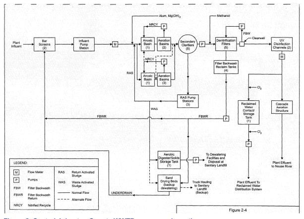
Figure 2. Central Johnston County WWTP process schematic.
