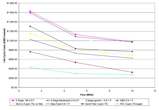
Figure 4-19. Life-cycle costs for expansion nitrogen plus phosphorus removal technologies.
