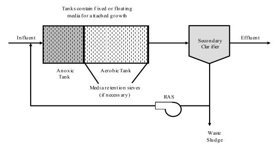
Figure 2-7. Integrated fixed-film activated sludge process.
