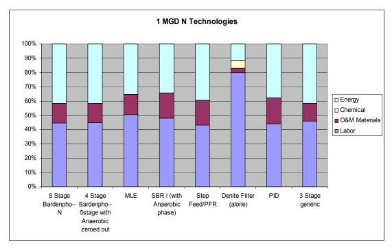
Figure 4-18. Component percentages of total O&M costs for 1 MGD expansion nitrogen removal technologies.
