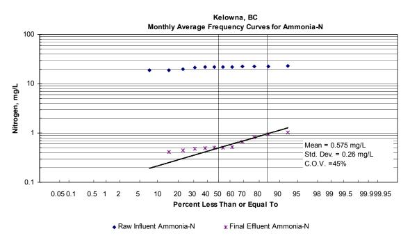
Figure 5. Monthly frequency curves effluent ammonia.
