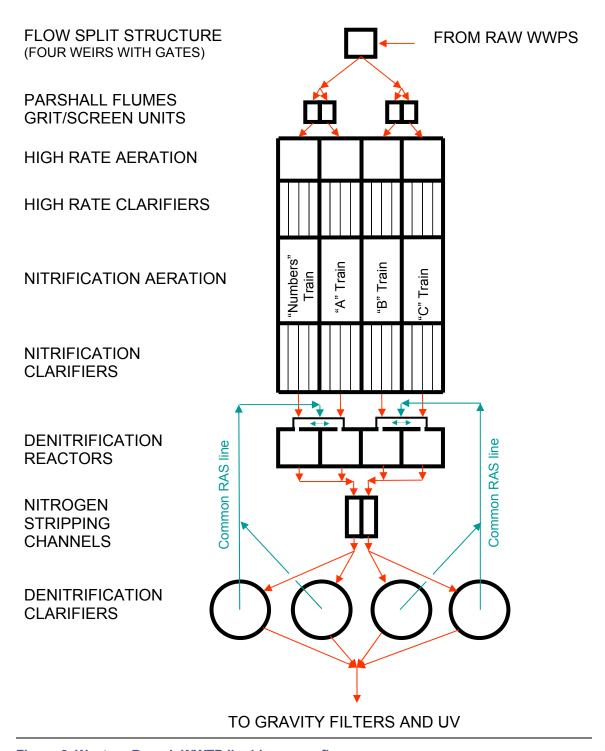
Figure 2. Western Branch WWTP liquid process flow.
