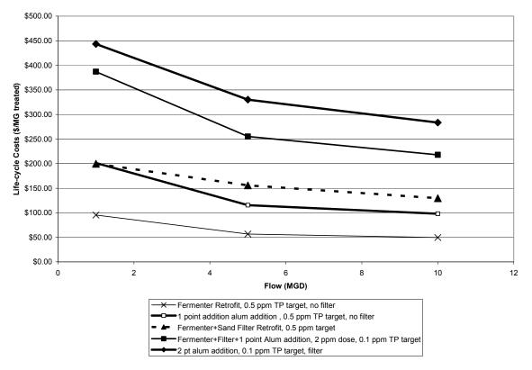
Figure 4-3. Life-cycle costs for retrofit phosphorus removal technologies (\$/MG treated).
