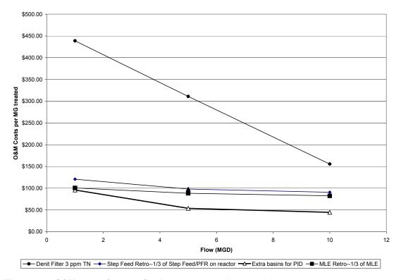
Figure 4-5. O&M costs for retrofit nitrogen removal scenarios.
