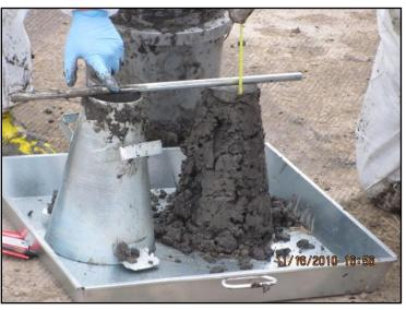
Photo 4-20. 2-Inch Slump Test of TSCA Material
