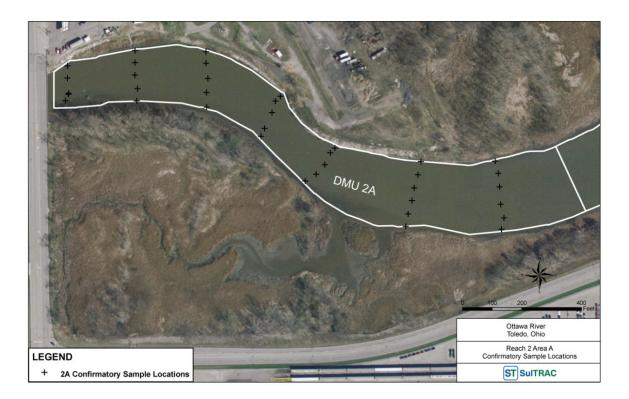
Figure 3-1. Example Confirmatory Sediment Sample Location Grid
