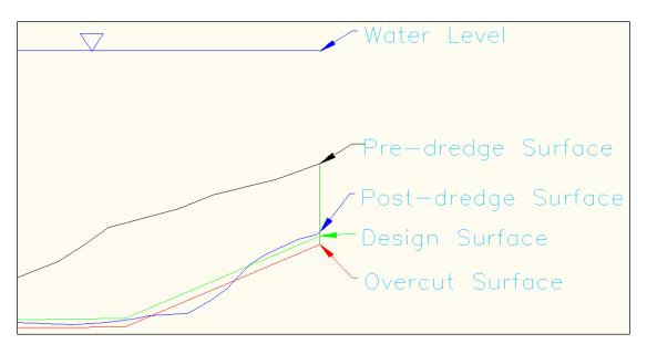
Figure 4-1. Example Cross Section
