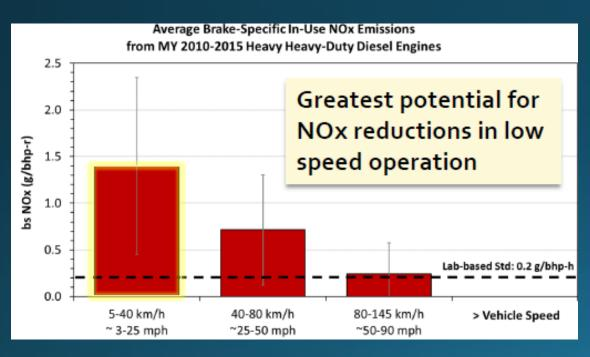
Data from 5 vehicles; all engines passed in-use testing standard of 0.3 g/bhp-h for conditions outlined in the test procedure
