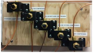
3. Turn the gas line valve to the "Closed" position (pointing down) for the gas to be changed.
